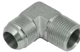
BSPP Male 60° Cone x JIC Male 90° Compact Elbow 37° Cone
