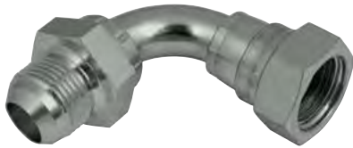
JIC Male 37° Cone x JIC Swivel Female 90° Swept Elbow
