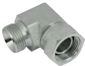
BSPP Male 60° Cone x JIC Swivel Female 37° Cone 90° Compact Elbow
